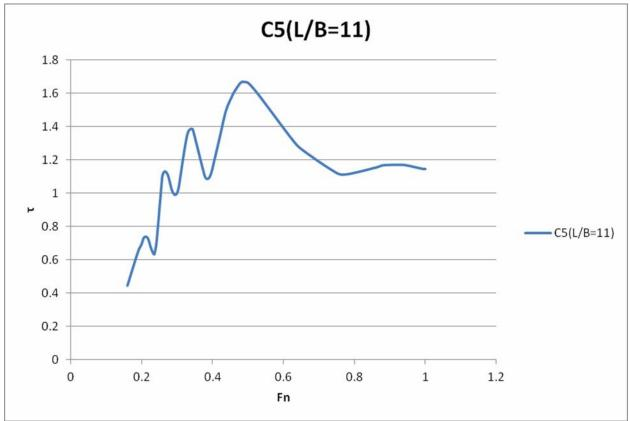
Figure 1: Wave interference factor,  $\tau$  Vs Froude no,  $F_n$ CONFIGURATIONS AND
